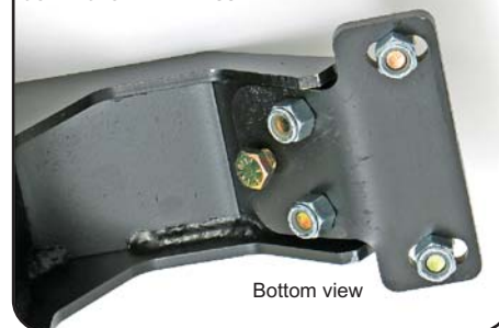
Illustration A CLOSE-UP OF FRAMERRAIL CONNECTOR PLATE ASSEMBLY
