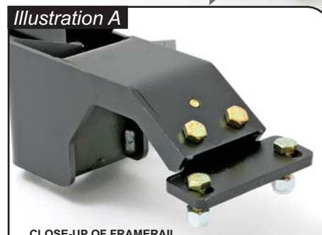
Illustration A CLOSE-UP OF FRAMERRAIL CONNECTOR PLATE ASSEMBLY
