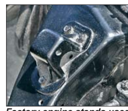
Factory engine stands used on 1970-71 Camaros
