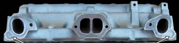
END BOLT HOLES MAY REQUIRE DRILLING & TAPPING
