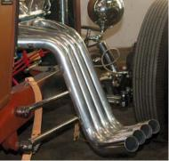
To ensure a proper seal, and to prevent exhaust leaks, install your newly built hedders using the Hedman Hedders gaskets included with this kit only, and a copper gasket sealant spray.
